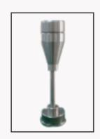
Abrasion head for pilling test
