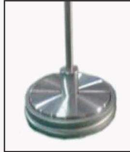
Abrasion head for pilling test
