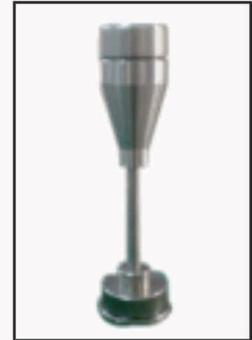
Abrasion head for abrasion test
