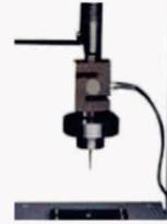
*test head for nail penetration*
